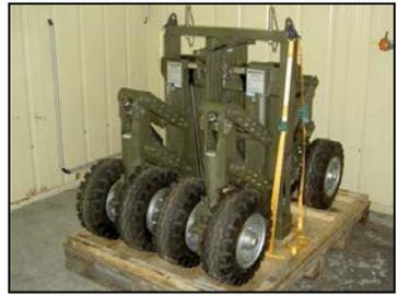
CDK Mobile Systems Inc. offers the Winglift Model W40 Mobilizer for short range handling and aircraft loading of ISO Containers, Tactical Shelters and Military Radar Platforms.
